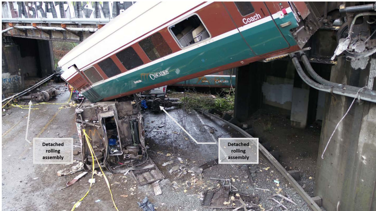
Figure 13. AMTK 7421 (11) resting on AMTK 7424 (8). (Photo provided by WSP.)
