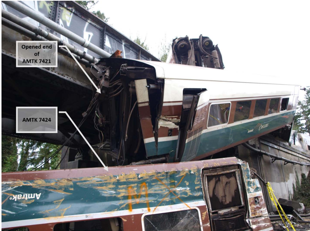
Figure 29. Open end of AMTK 7421 (11). (Photo provided by WSP.)
