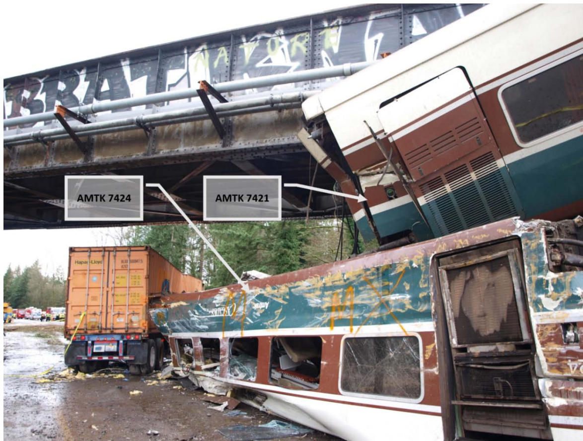
Figure 28. AMTK 7421 (11) resting on AMTK 7424 (8). (Photo provided by WSP.)
