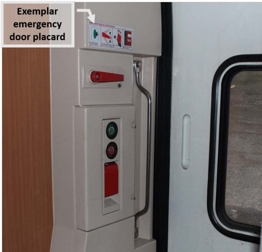
Figure 37. Exemplar emergency door showing instruction placard.
